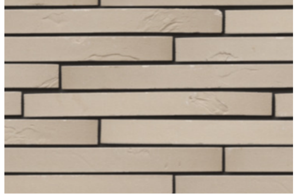
Archipolis Byblos Grey Eco-brick ± 400x65x40 mm Porosity: ≤ 6% IW1 - very low absorption
