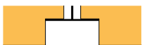
Shiplap edges RDT for thicknesses 25 - 35 mm with T24 profile RDT35 for thicknesses 25 - 35 mm with T35 profile
