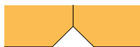
Chamfered edges S4 for CELENIT L2ABE25C and CELENIT L2ABE25C/A2 boards S47 for CELENIT L2AB - CELENIT L2ABE/A2 - CELENIT L2AB/A2 boards
